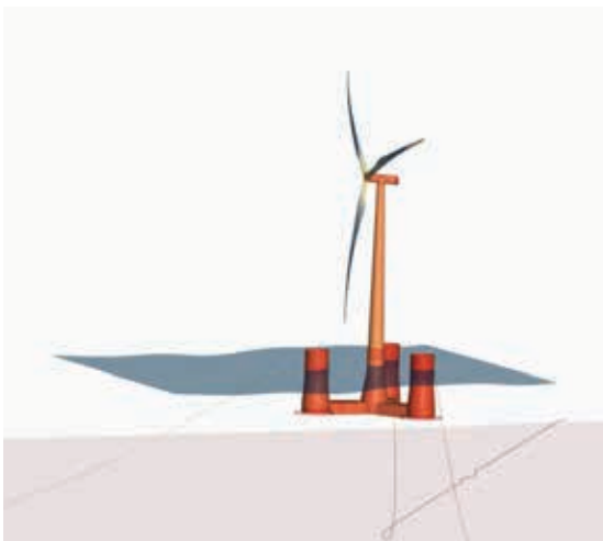
Figure 15: 3DFloat simulations of Dr.techn Olav Olsen's 6 MW concrete semi-submersible offshore wind turbine.
